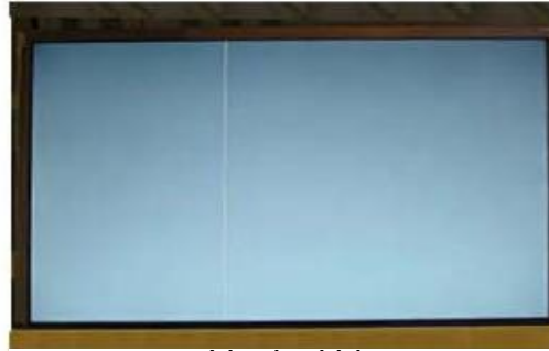
Vertical Line Source TAB IC Defect
