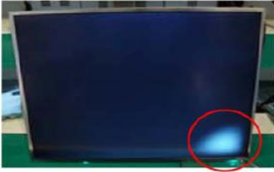
Panel Mura, Light leakage
