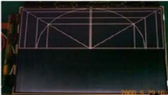
Horizontal Block Gate TAB IC Defect
