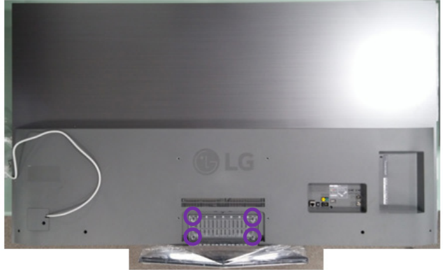
(3) Remove Stand Screw and Stand
