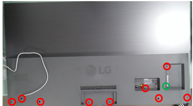
(4) Remove Back Cover Screw
