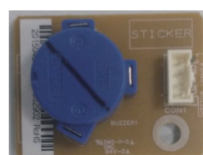
Buzzer PCB ( P/N : EBR76332902 )
