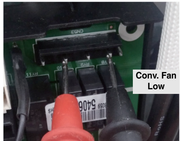
3th pin and 7th pin of CN53 : RY 9
