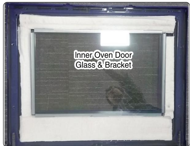
**REASSEMBLY NOTE:** When you reinstall the insulation around the oven door glass, make sure that the insulation is not visible in the glass after the door is reassembled.
