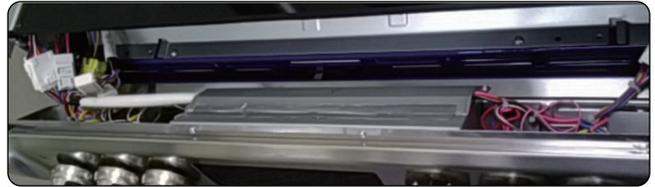
You can remove the controller after unplug the 7ea connectors of Main PCB and Cooktop
