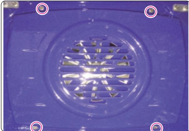
6. Remove the two convection element screws and pull the element forward.
