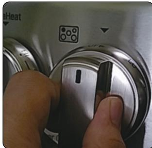
c) Remove the 2 screw of Knob Housing
