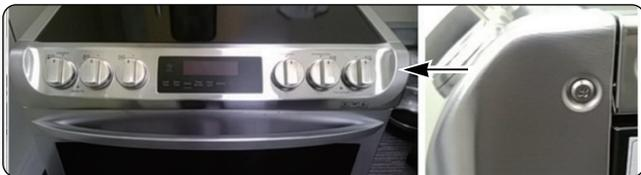
4. Remove the 4 screws located under the controller.
