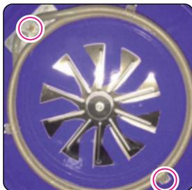
7. To remove Fan blade, remove Nut by screwing clockwise. Fan blade can be replaced from inside oven.
