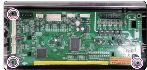
5. To remove the Key PCB assembly remove the 2 screws under the controller.
