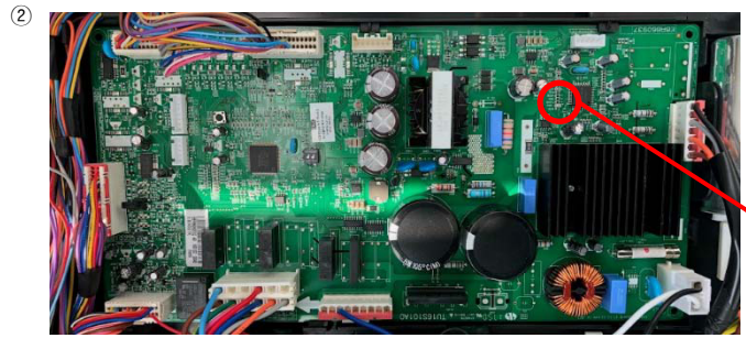
2. Check the number of LED blinks (Refer to the next page for resolution by number of LED blinks)
