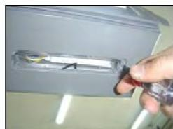
4. Remove the LED assembly from connector.
