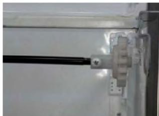
Step 4) Insert opposite gear ice into connector rail and screw them
