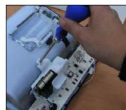
3) Disconnect wire harness from wall of compartment.
