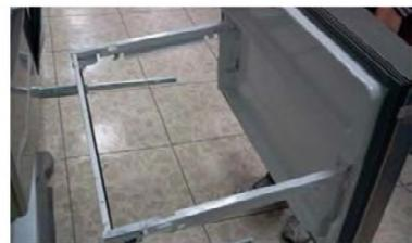
Step 5) Remove only 1 screw of gearice, and disassemble the bar and gearice
