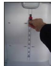
3. Disconnect the lead wire on the bottom position
