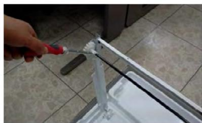
Step 6) Remove 2 screws of both side of supporter covers tv and disassemble the supporter cover tv.
