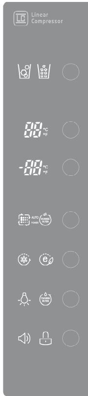
\* Display check function: If simultaneously pressing Ultra Ice button and freezing temperature adjustment button for a second, display LCD graphics on. If releasing the button, the LCD graphic displays the previous status.
