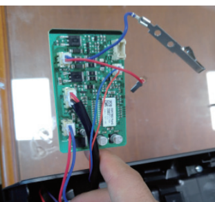
(7) Remove the harness connector and replace the PCB.
