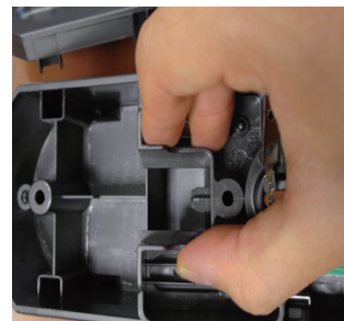
(6) Remove the bump inside the terminals and take out the PCB.
