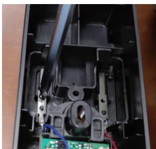
(5) Remove the terminals of the charging station.
