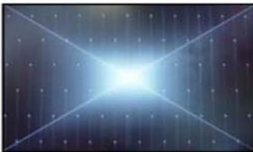
Solder defect, Short/Crack
