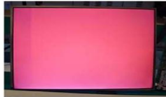
Vertical Block Source TAB IC Defect
