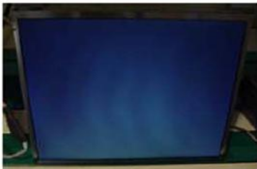
Panel Mura, Light leakage
