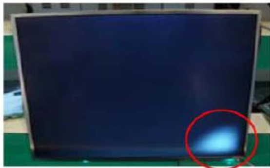
Panel Mura, Light leakage
