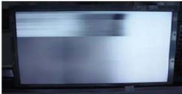
Horizontal Block Gate TAB IC Defect
