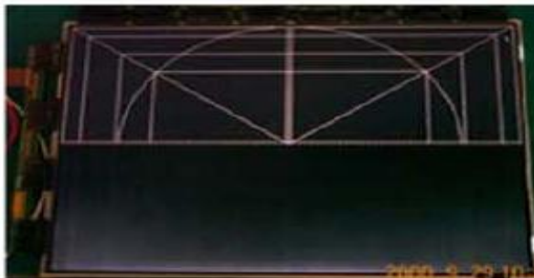
Horizontal Block Gate TAB IC Defect
