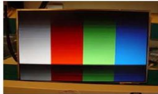
Horizontal Block Gate TAB IC Defect
