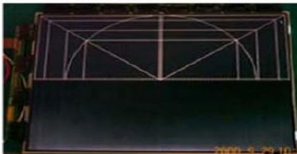
Horizontal Block Gate TAB IC Defect
