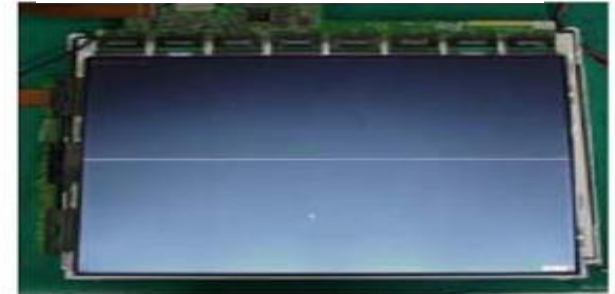
Horizontal line Gate TAB IC Defect
