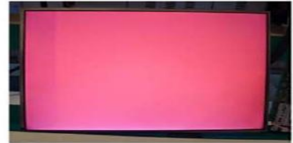
Vertical Block Source TAB IC Defect
