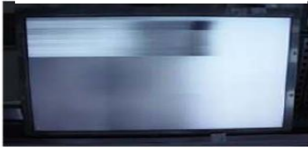
Horizontal Block Gate TAB IC Defect
