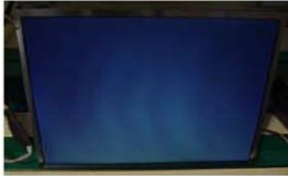
Panel Mura, Light leakage
