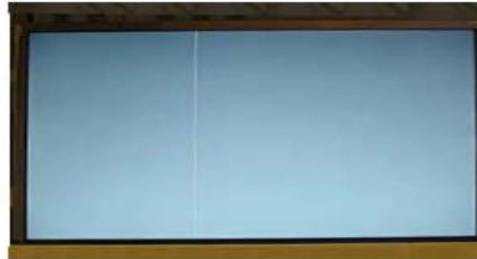
Vertical Line Source TAB IC Defect
