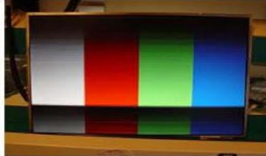
Horizontal Block Gate TAB IC Defect
