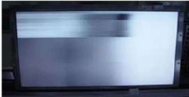
Horizontal Block Gate TAB IC Defect
