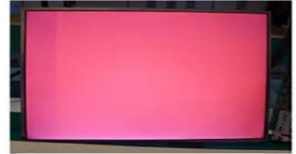
Vertical Block Source TAB IC Defect
