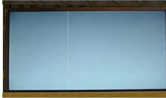
Vertical Line Source TAB IC Defect
