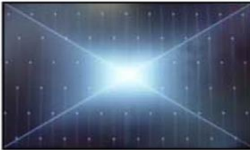
Solder defect, Short/Crack
