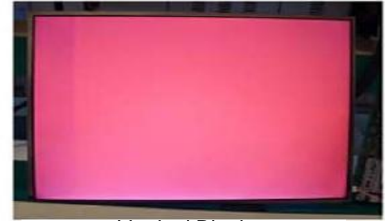
Vertical Block Source TAB IC Defect
