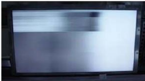
Horizontal Block Gate TAB IC Defect
