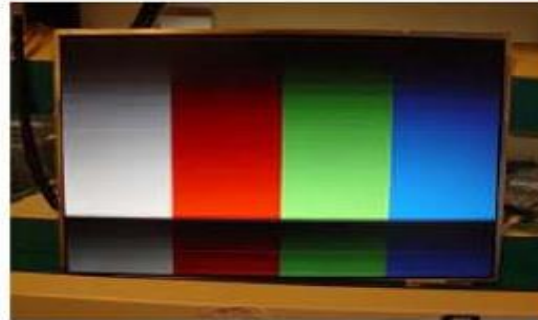
Horizontal Block Gate TAB IC Defect
