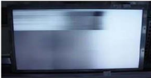
Horizontal Block Gate TAB IC Defect
