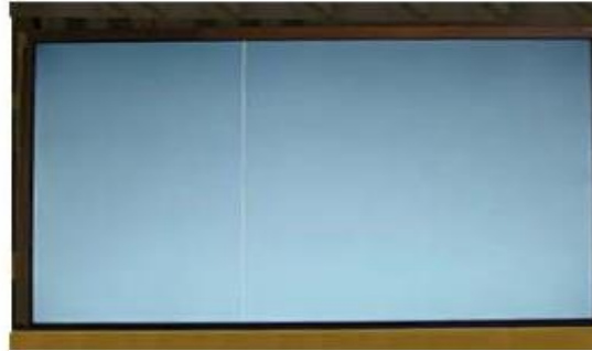
Vertical Line Source TAB IC Defect
