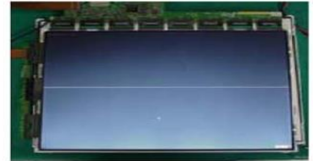
Horizontal line Gate TAB IC Defect
