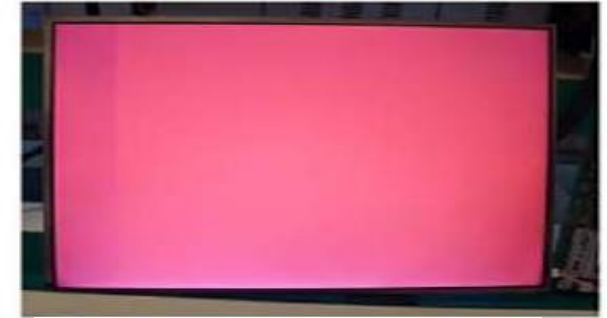
Vertical Block Source TAB IC Defect
