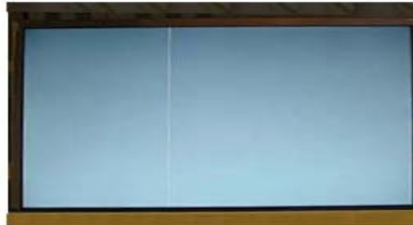
Vertical Line Source TAB IC Defect
