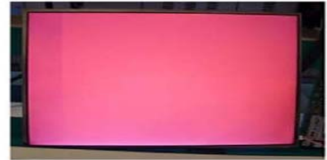
Vertical Block Source TAB IC Defect
