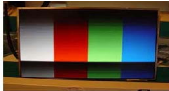
Horizontal Block Gate TAB IC Defect
