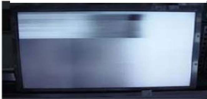
Horizontal Block Gate TAB IC Defect
