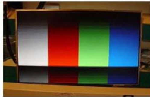
Horizontal Block Gate TAB IC Defect
