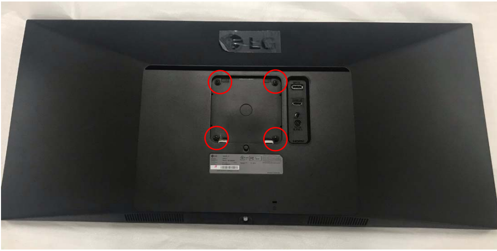
Fig 3 Remove the Screw(4EA) and disassemble the back cover
