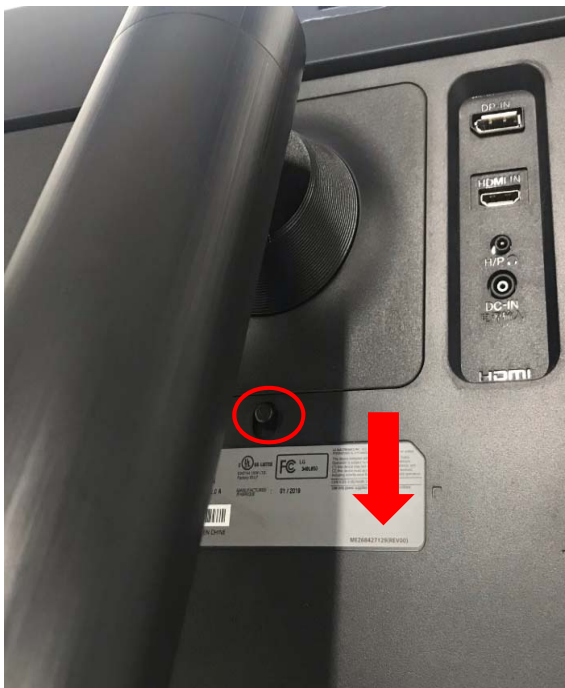
Fig.2 Disassemble the Stand body with pulling down the button.
