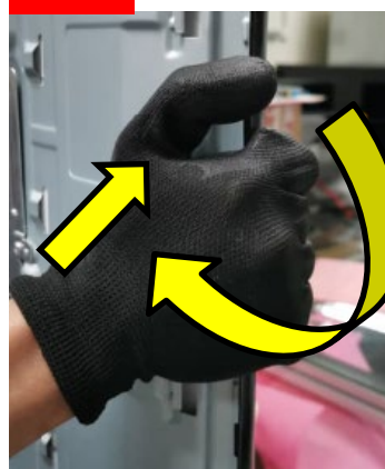
Since the O-cell may pop out, DO NOT apply force to the Back Chassis or rotate the Bezel
