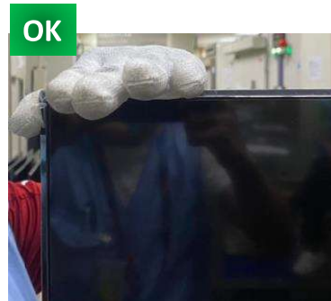
Holding edge of Bezel without touching O-cell
