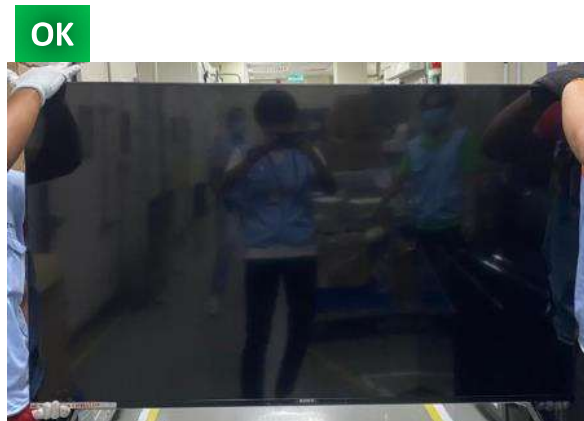
Always wear gloves during P-mod handling
