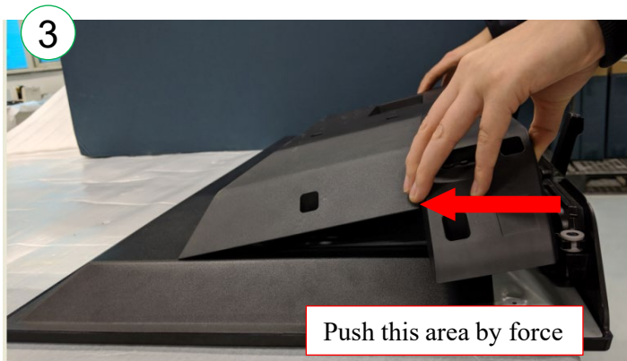
3. Push the rear cover as picture shown to release the hooks. (Be careful the keypad FFC wire)
