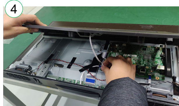
4. Flip up the rear cover as picture, remove keypad FFC wire.
