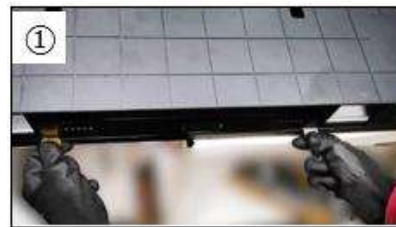
Locate both hooks and unhook using coin/Jig.
