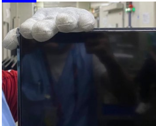
Holding edge of the Bezel without touching the O-cell
