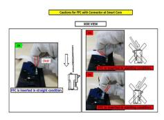
\* Do not push hard on FFC connector on H Board to avoid connector peel off
