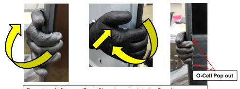
Do not apply force on Back Chassis and rotate the Bezel → Can cause O-cell to pop out
