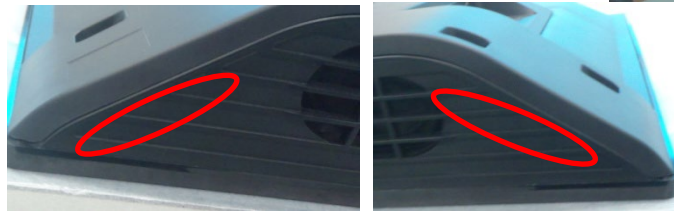
1. Push both side of the front bezel corner area (show as the picture) and the hook- opening voice can be heard .
