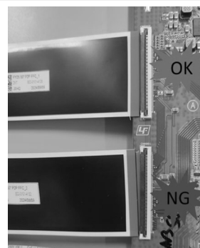
CAUTION FOR FFC WITH CONNECTOR INSTALLATION AT MB SIDE
