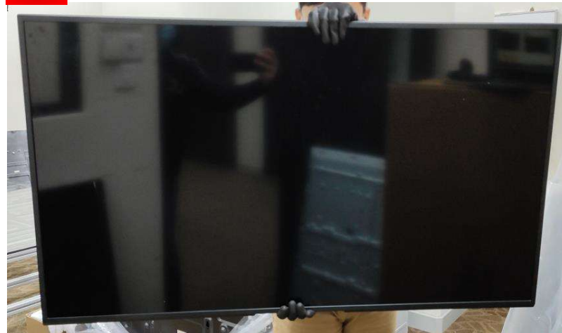
Carry P-mod at center area
