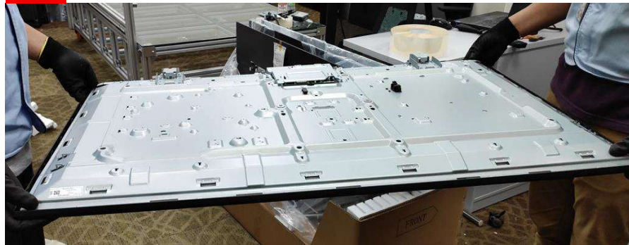
Carry P-mod by Horizontal position
