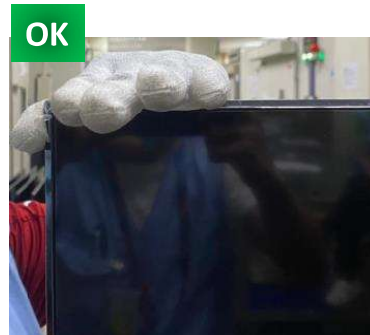
Holding edge of Bezel without touching O-cell
